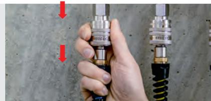
Disconnection – second step: pressureless disconnection
