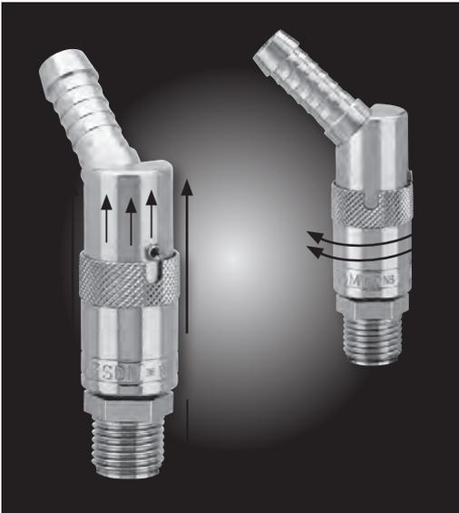
Sleeve locking mechanism offers a simple and effective prevention in respect of unintended disconnection under pressure due to a pin sleeve lock design (pin/notch)
