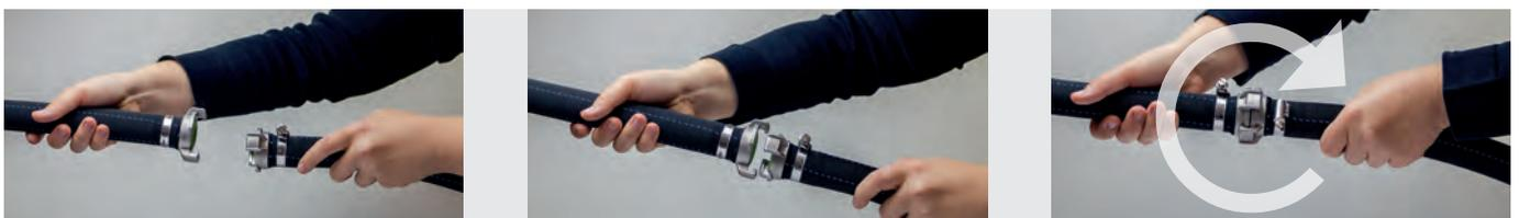
The principle of connecting is identical with the functioning of the WaterProfi Claw Couplings. Both couplings are connected at the front end side in order to connect the sealing surfaces. Afterwards one coupling half has to be twisted against the other until end stop – the plug locks into place.
