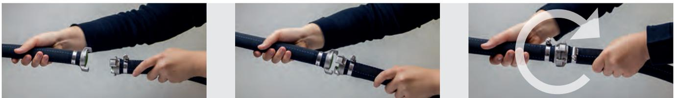
The concept of connecting is identical with the functioning of the WaterProfi Claw Couplings. Both couplings are connected at the front end side in order to connect the sealing surfaces. Afterwards, one coupling half has to be twisted against the other until end stop – the plug locks into place.
