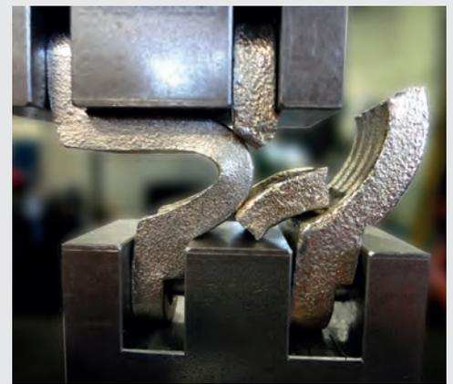
Distance of 23 mm (completely destroyed counterfeit, no cracks in the **LUDECKE** hose clamp)
