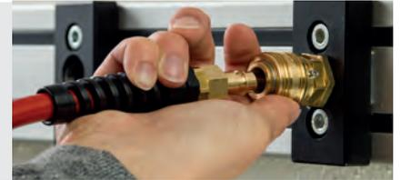
DN 7.2: to disconnect, the locking pin has to lock exactly into the sleeves milling when the sleeve is pulled back
