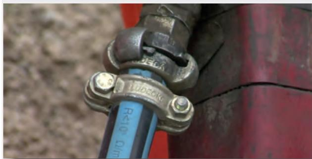
The **LUDECKE** success story started with the development of claw couplers. To date, this coupling type is used worldwide in various compressed air applications in the industrial and construction industry.
