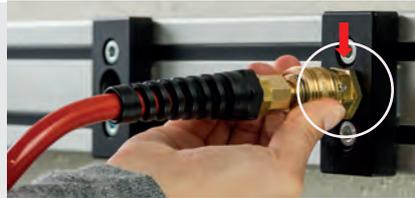
Securing through twisting of the sleeve
