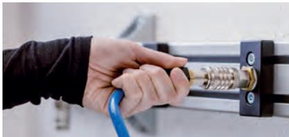
One-hand operation, additional locking feature due to screw lock on coupling body – mechanical lock with counter (pinch) screw
