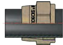
Also move the slotted squeeze ring with the cone ahead over the hose which must be cut to straight length. Make sure that the edge of the ring (labelled with the corresponding hose dimension) is flush with the hose's end.
