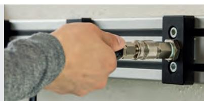
Two-hand operation: To disconnect push the plug into the coupling, then the locking mechanism works.
