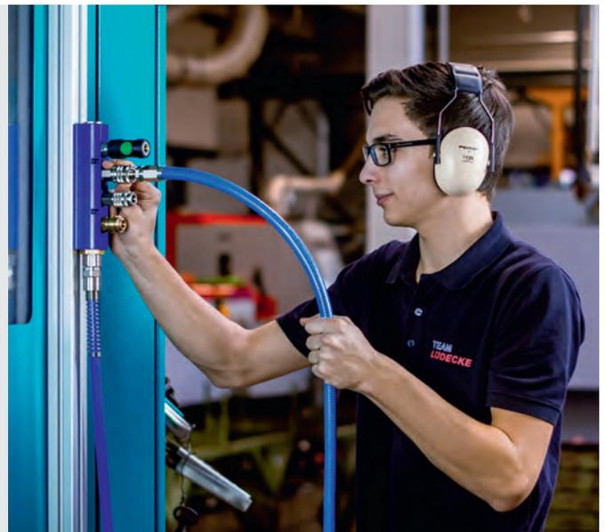
Whiplashing effect: high risk of injury in the usage of compressed air – avoidable through the use of products from the **LUDECKE SafeConnect-Line**.
