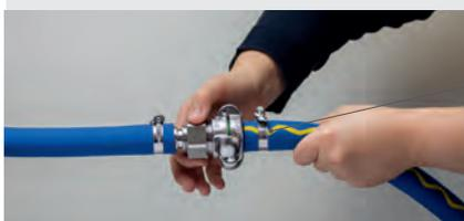
To ensure a proper locking, the MODY safety screw type coupling is locked with an additional locking nut underneath the claw head.
