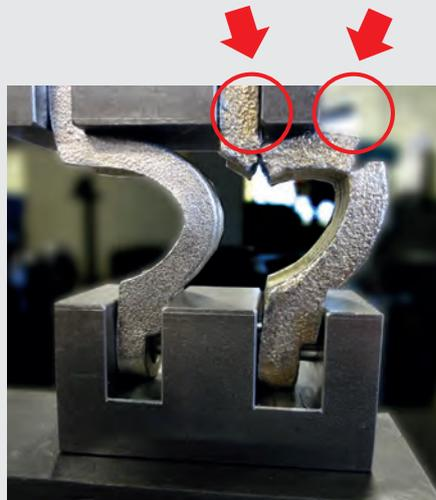
Distance of 28 mm (complete break in the counterfeit, no rupture in the **LUDECKE** hose clamp)
