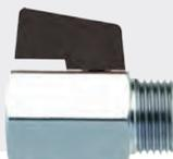
Ball-Valves serve as shut-off fittings in pipe-systems for compressed air and other media. They seal through PTFE-shells and are especially suited for use in industrial installations.
