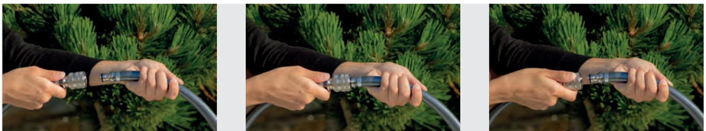
To disconnect, grasp the plug firmly with one hand. With the other hand push the locking sleeve backwards and pull the plug off the coupling. After disconnecting, the locking sleeve slips automatically back to starting position. This system allows not only a fast work process, but also a reduction to a minimum of potential injuries in term of finger trapping etc.
