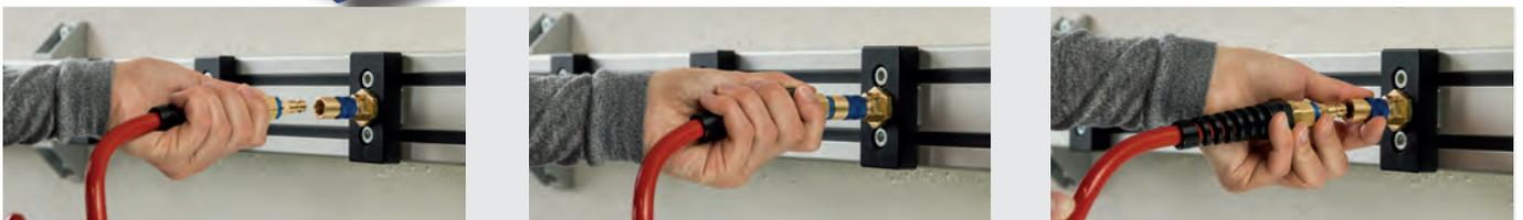
One-hand operation: connection via pushing of the plug into the coupling. Thereby, the colours of the sleeve of aluminium of the coupling and the ring of aluminium of the plug as well as the plug- coding have to be identical.
