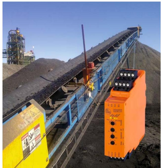
Use for rotational speed monitoring on conveyor belts, worm gears and elevators.
