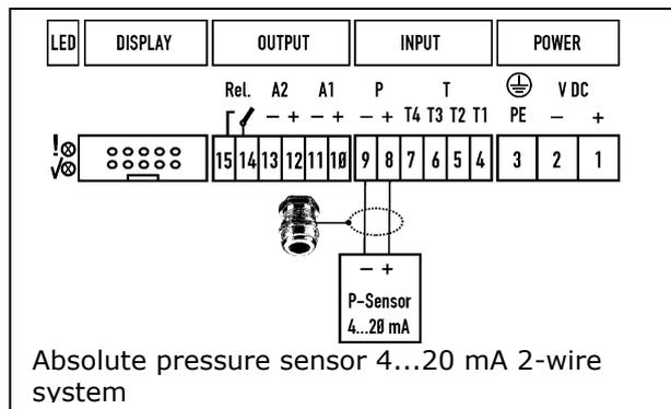
The initial value (4 mA) and the terminal value (20 mA) can be configured with the PC software UCOM via the RS232 interface. Customer-specific programmed values can be found in the accompanying documents.
