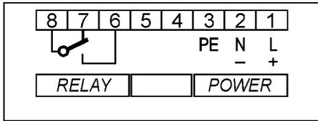
The normally open contact is shown in rest position (relay coil off).
