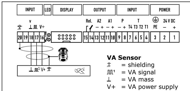
In the case of sensor housings with screwed cable glands, the shielding of the sensor connection cable is connected in the cable glands.
