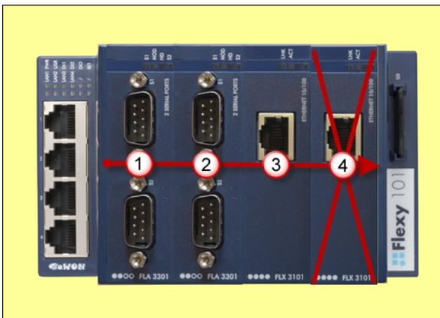
Example of configuration that would be OK mechanically and power wise, but that is not supported by the firmware.
