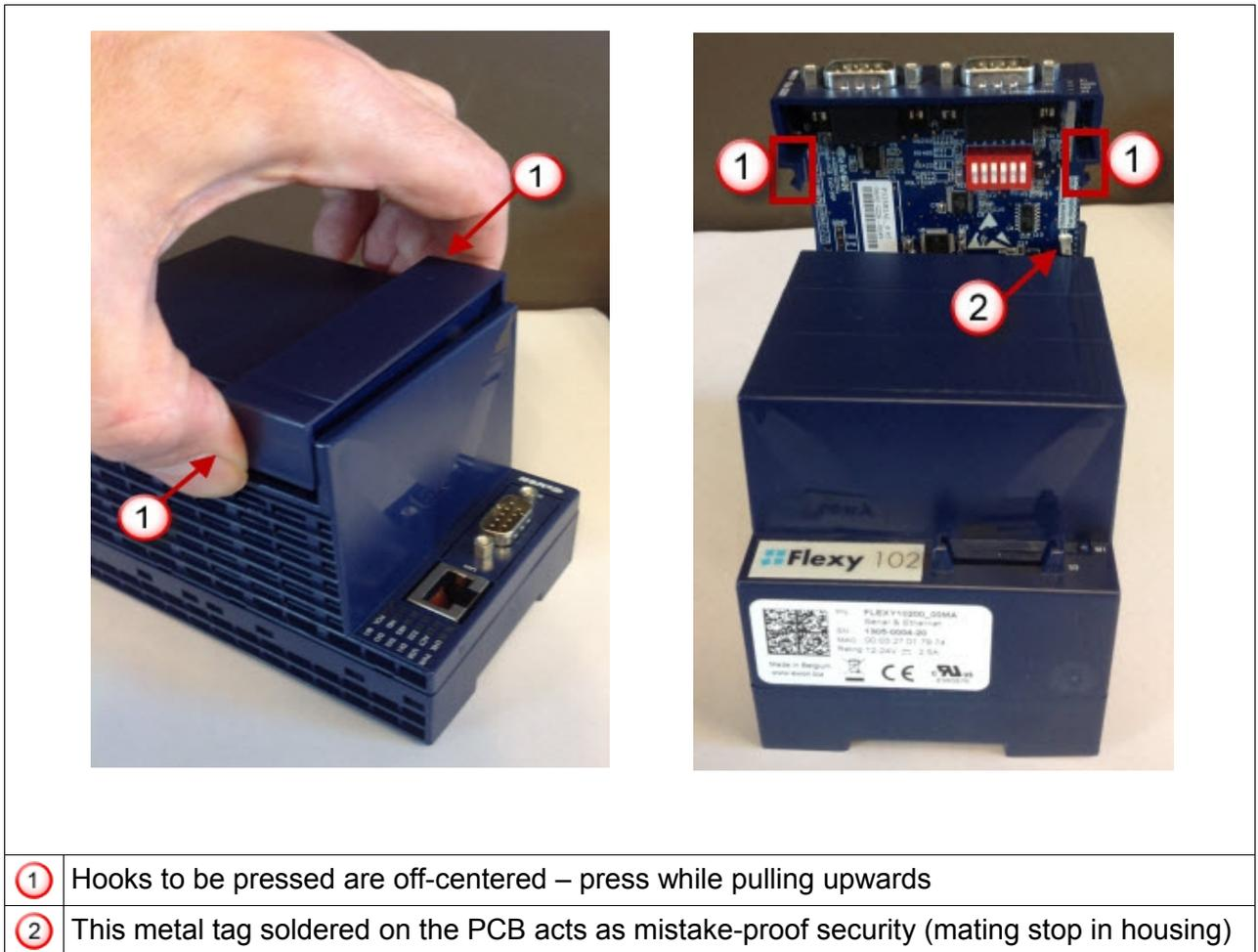
Insert the Extension Card carefully and slide it down until the hooks are **clicking**. Make sure the card is completely inserted. **DO NOT insist** if you feel some resistance when trying to insert the card. It probably means you are trying to insert a card in a wrong slot. In such case, check slot compatibility of the relevant Extension Card. Refer to § 4.1 Base Unit Slot Compatibility.
