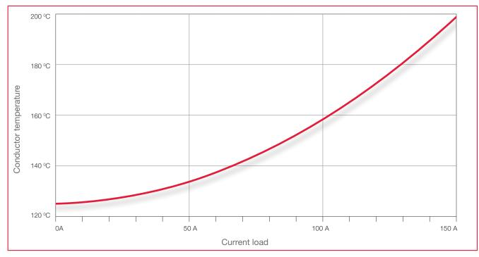
This type of derating curve can apply to only one environment temperature at a time. The curve shown above starts with an environment temperature of +125 °C.
