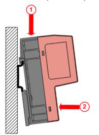
Push the device onto the top hat rail from above 1.
