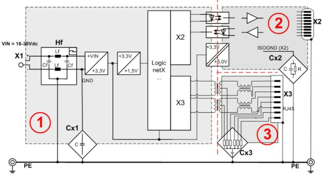
Figure 6: netTAP NT 50-MPI, Coupling
