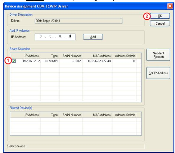
Step 5D: Connect the system configurator SyConMPI with the MPI device:
