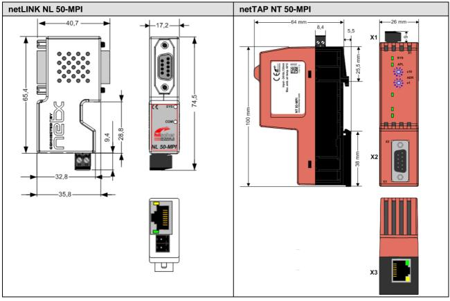
Figure 1: Dimensioned Drawing NL 50-MPI and NT 50-MPI (Size in mm)
