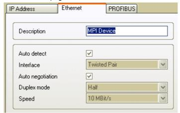
Figure 26: Ethernet Parameters are detected automatically by the MPI Device
