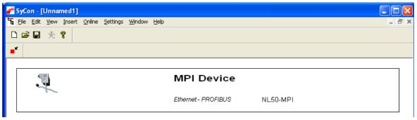
Figure 24: System Configurator SyConMPI – The MPI Device is displayed in the Project
