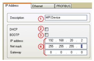
Figure 41: Settings > MPI Device Parameter > IP Address
