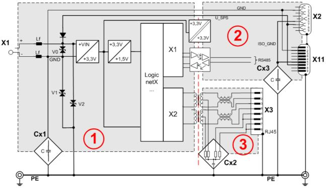
Figure 5: netLINK NL 50-MPI, Coupling (Hardware Revision 4)
