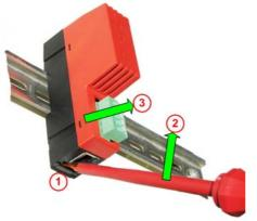
To release the device from the tophat rail, use a screw driver, which you put at the clip 1 in the center of the device. By pressing slightly the screw driver in direction of arrow 2 the lock at the top-hat rail is released. You can then easily pull the device off the top-hat rail in direction of arrow 3.
