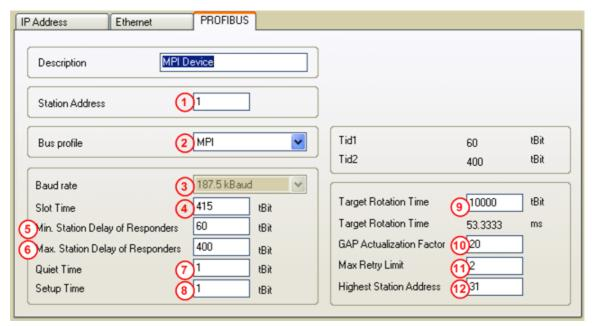
Figure 43: Settings > MPI Parameters > PROFIBUS
