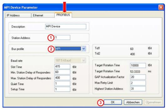
Figure 27: Set the PROFIBUS Parameters
