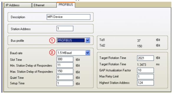
Figure 44: Settings > MPI Parameters > PROFIBUS > Autobaud
