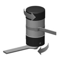
3. Examine bottom section, especially sealing surfaces, for mechanical damage.
