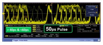
DPO70000SX includes a unique Envelope trigger mode that enables direct triggering on the envelope of a modulated carrier. Edge, Width and Timeout trigger types can be applied to a detected envelope to provide stable trigger on modulated bursts or discriminate bursts of a specific width. Carrier frequency can range from 500 MHz to 20 GHz to address a broad range of applications. The figure illustrates triggering on burst of specific width.
