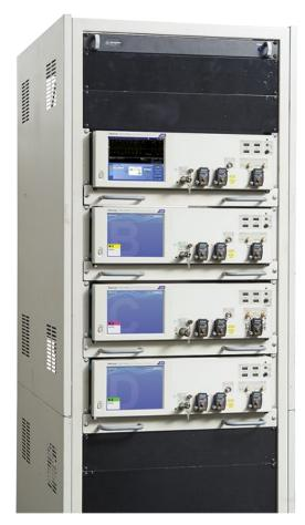
The rack-mounting kit allows units to be mounted upright or inverted to minimize input cable length, just as when stacking on a bench.
