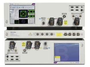
DPO70000SX units may even be operated inverted if desired, to shorten OMA receiver connection distance as shown.
