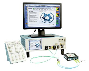
SignalCorrect allows quick characterization of cables, fixtures and other types of interconnects using the TCS70902 fast step source and the response captured on a DPO70000SX Series real-time oscilloscope.
